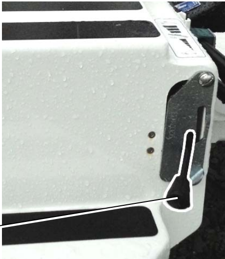
Fig. 1-3-8-3: Mechanic hand throttle lever
