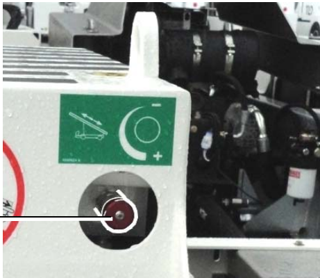
Fig. 1-3-8-1: Hydraulic hand throttle wheel
